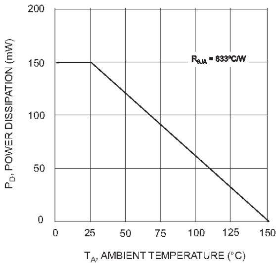
Fig. 1 Derating Curve
