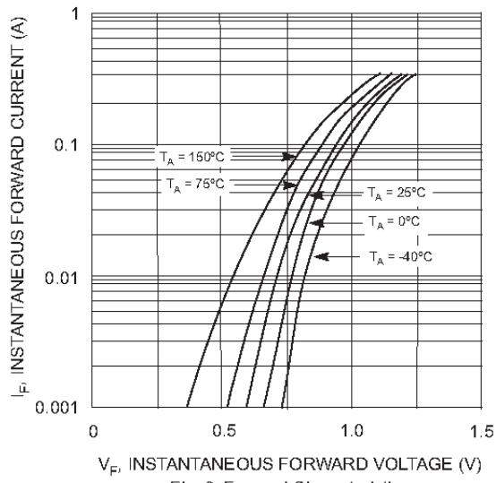
Fig. 2 Forward Characteristics
