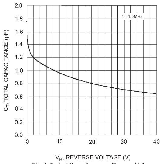
Fig. 4 Typical Capacitance vs. Reverse Voltage
